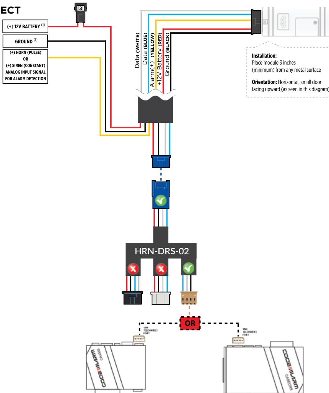
(1) Connect to supply power to telematics device
